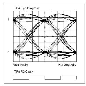
Clearly the goodness of this convergence is an indication of the way the modem will perform. Vertical scatter at the sample point reduces the system's tolerance to noise, because some bits pass closer than others to the mid-screen decision threshold. This scatter is "self-noise", and adds to any real noise present.
